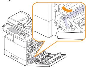
Carefully remove the misfed paper in the direction shown.
